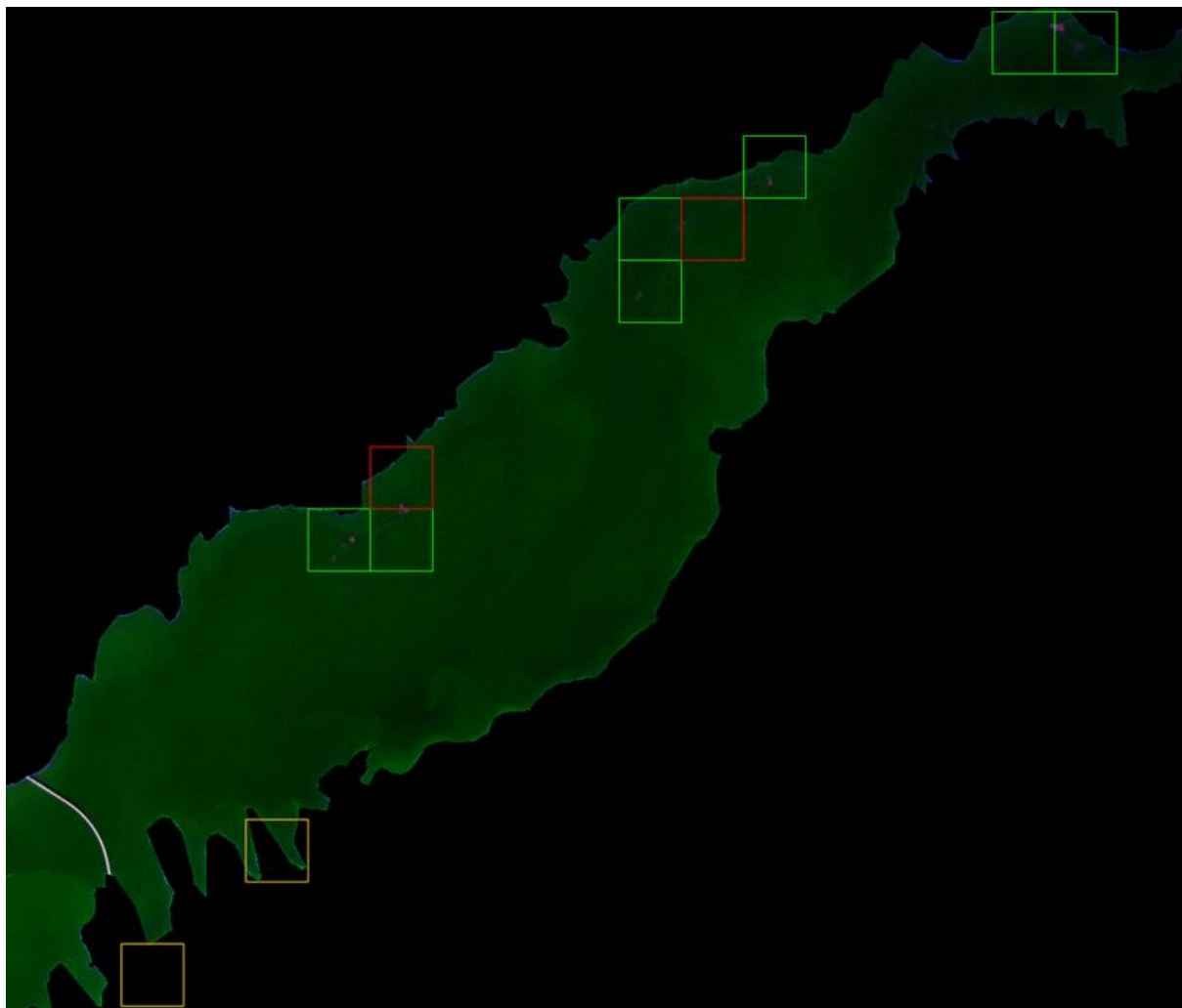
Figure 16. Output of the oil spill prediction module on product S2B_MSIL2A_20171230T092359_N0206_R093_T34TEK_20171230T115949. With green the true positives. With red the false negatives. With yellow the false positives.
